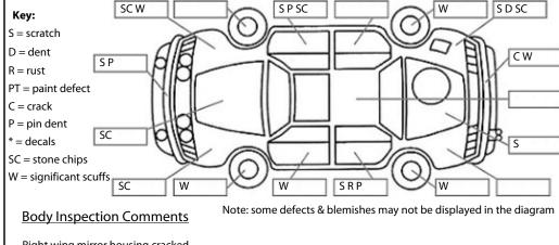
Right wing mirror housing cracked Rear bumper misaligned
