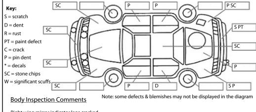
Right wing mirror indicator lens cracked. Stone chip on windscreen
