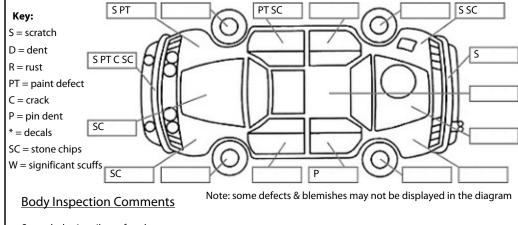
Screw holes in tailgate for plate. Screw holes in bumper. Left spotlight cover missing
