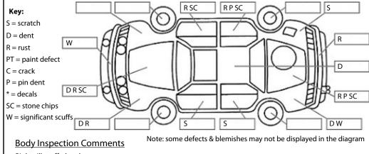
Right sill scuffed and rust Left running board cracked Rusty tow bar
