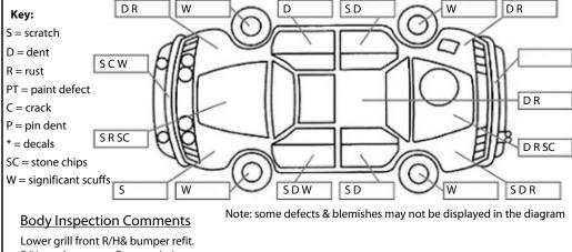
Lower grill front R/H& bumper refit. R/H rear bumper reflector missing. L/H sliding door not flush when closed. Windscreen chip.
