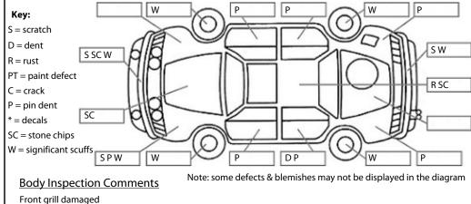
Front grill damaged Left rear door doesn't open
