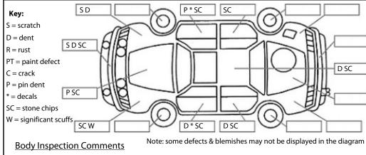
Running boards bent. Right cant rail dented. Rear panel on deck bent. Rear mud guards bent. Chipped windscreen
