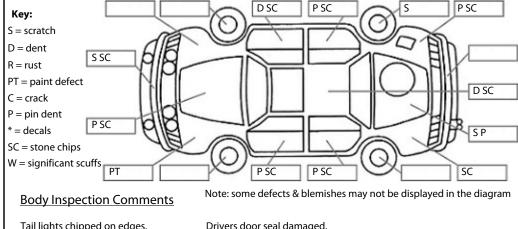
Tail lights chipped on edges. Drivers door seal damaged. Cab corners pin dented. Chipped windscreen.
